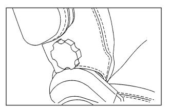
If your vehicle has this feature, turn the knob located on the driver's side seatback to adjust support of the lower back.
